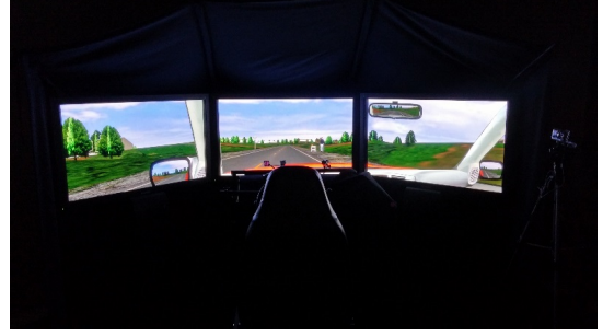
Fig. 1: Simulator setup - National Advanced Driving Simulator (NADS) MiniSim with three screens.
